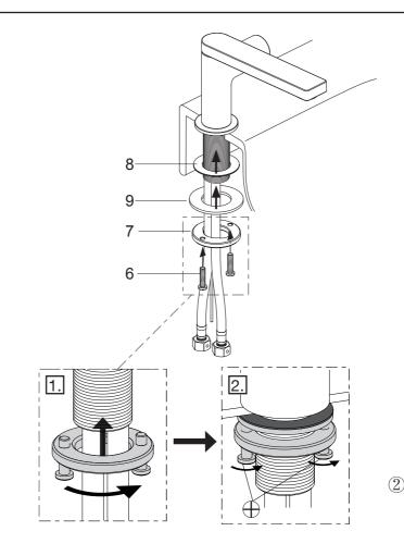
From underside of the basin, place the washers(8, 9) onto the shank.
